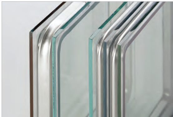
Double and triple glazed windows deliver outstanding thermal performance. Low conductivity warm edge spacers keep the panes of glass apart.
